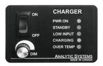
A remote control panel may be connected to the converter using a 9-pin D-connector, which attaches to the side of the converter. The remote control panel and D connector are part of the remote control option. The remote control panel allows the unit to be operated remotely as well as duplicating all the diagnostic indicators and audible alarm.
