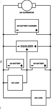
It is recommended to keep all wiring as short as possible to keep the line losses to a minimum.
