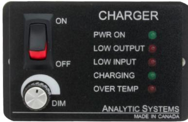
A remote control panel may be connected to the converter using a 9-pin D-connector, which attaches to the side of the battery charger. The remote control panel and D connector are part of the remote control option. The remote control panel allows the unit to be operated remotely as well as duplicating all the diagnostic indicators and audible alarm.
