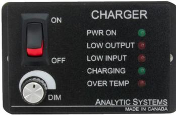
A remote control panel may be connected to the battery charger using a 9-pin D-connector, which attaches to the side of the battery charger. The remote control panel and D connector are part of the remote control option. The remote control panel allows the unit to be operated remotely as well as duplicating all the diagnostic indicators and audible alarm.
